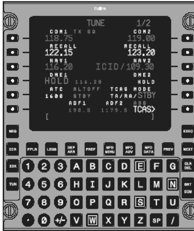
Fig. 5 - Control Display Unit (CDU)
